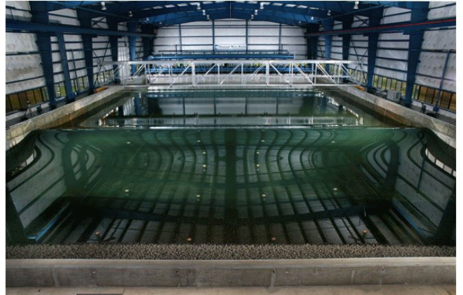
Fig. 6. Directional wave basin at Oregon State University.
